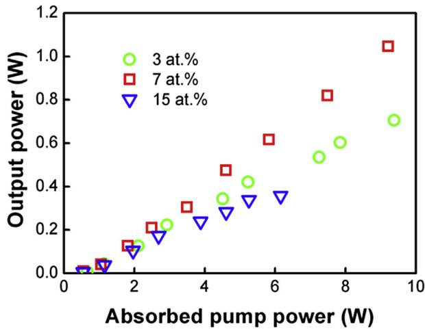
Fig. 3. Output powers versus absorbed pump power for Er:Y<sub>2</sub>O<sub>3</sub> ceramic samples of 3 at.%, 7 at.%, and 15 at.% Er<sup>3+</sup> concentration.
