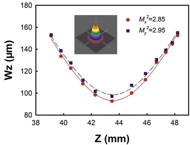
Fig. 5. Beam quality of the 2.7 μm Er:Y<sub>2</sub>O<sub>3</sub> ceramic laser under ~19.6 W of absorbed LD pump power.
