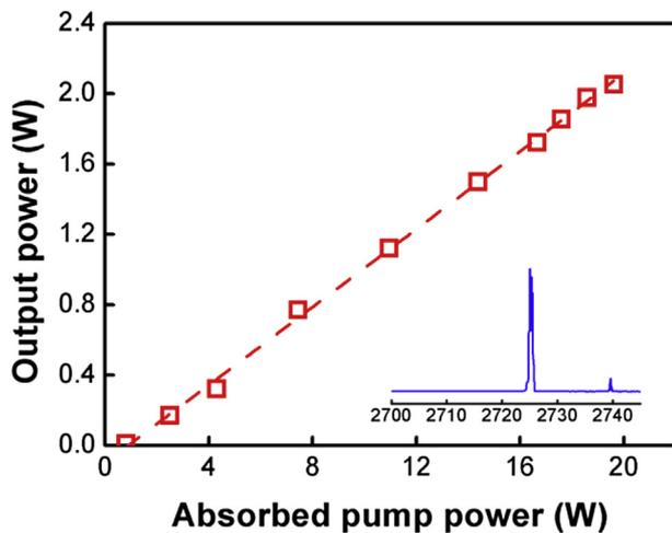
Fig. 4. Laser output powers versus absorbed pump power for the 7 at.% concentration Er:Y<sub>2</sub>O<sub>3</sub> ceramic sample. Inset: output spectrum of the ceramic Er:Y<sub>2</sub>O<sub>3</sub> laser at 2.7 μm.
