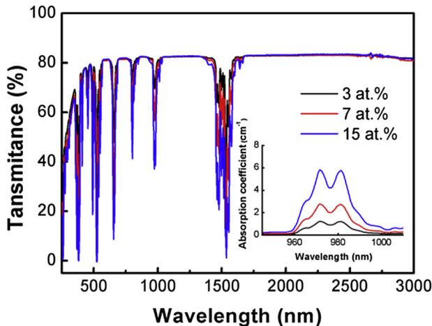
**Fig. 1.** Transmittance spectra of 1.33 mm thick Er:Y<sub>2</sub>O<sub>3</sub> ceramic samples with 3 at.%, 7 at.%, and 15 at.% Er<sup>3+</sup>-doping concentration. Inset: absorption spectra of the Er:Y<sub>2</sub>O<sub>3</sub> ceramics in the region of Er<sup>3+</sup> <sup>4</sup>I<sub>15/2</sub> absorption.
