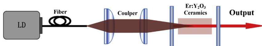
**Fig. 2.** Experimental setup for LD end-pumped Er:Y<sub>2</sub>O<sub>3</sub> ceramic lasers.
