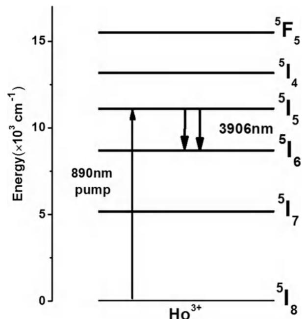
Fig. 2. The simplified energy level diagram of  $Ho^{3+}$  doped YAP crystal.
