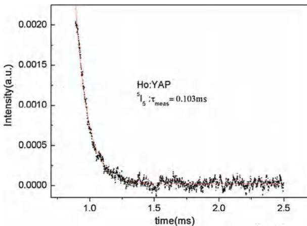
Fig. 4. The fluorescence decay curve of the  $^5I_5$  level in Ho:YAP crystal at room temperature.
