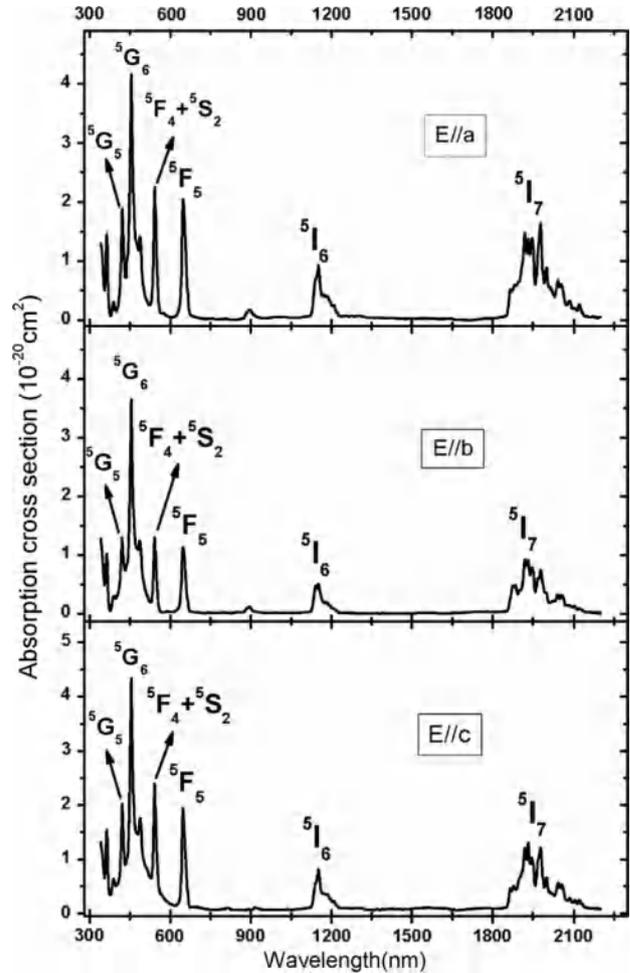
Fig. 1. Polarized absorption spectra of Ho:YAP crystal at room temperature.
