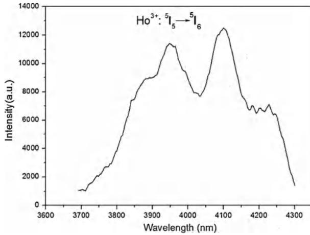
Fig. 3. Fluorescence spectrum of Ho:YAP crystal in the wavelength of 3700–4300 nm.
