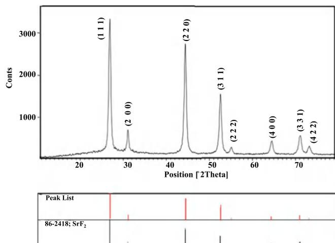
Fig. 1. XRD pattern of SrF<sub>2</sub> phosphor.
