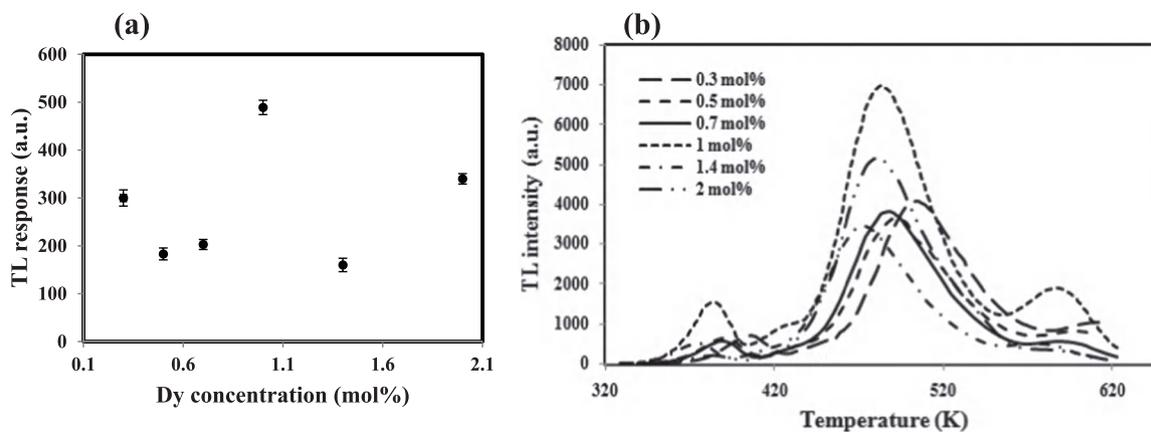
Fig. 3. TL responses for different dysprosium concentrations in SrF<sub>2</sub>:Dy phosphor (a) and the corresponding TL glow curves (b) after 5 Gy gamma irradiation.
