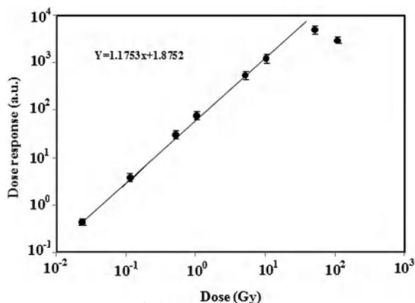
Fig. 4. Dose response of SrF<sub>2</sub>:Dy sample.
