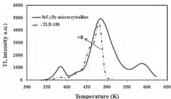
Fig. 5. Comparison of TL sensitivities of SrF<sub>2</sub>:Dy powder and LiF:Mg,Ti (TLD-100) after 1 Gy gamma irradiation. TL glow curve of TLD-100 was enlarged by a factor of 8 for better presentation.
