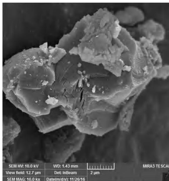
Fig. 2. SEM images of the produced SrF<sub>2</sub>:Dy phosphor.
