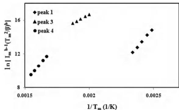
Fig. 8.  $\ln [I_m^{b-1}(\frac{T_m^2}{\beta})^b]$  against  $\frac{1}{T_m}$  for different glow peaks of SrF<sub>2</sub>:Dy phosphor. The slope of each line is equal to  $\frac{E}{k}$ .
