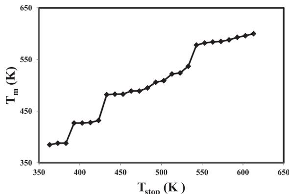
Fig. 6. Variation of peak maximum (T<sub>m</sub>) versus T<sub>stop</sub> for the produced SrF<sub>2</sub>:Dy phosphor.
