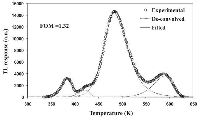
Fig. 7. Experimental TL glow curve (hollow circles), fitted glow curve (solid curve) along with component glow peaks (dashed curves) for the SrF<sub>2</sub>:Dy for absorbed dose of 5 Gy.
