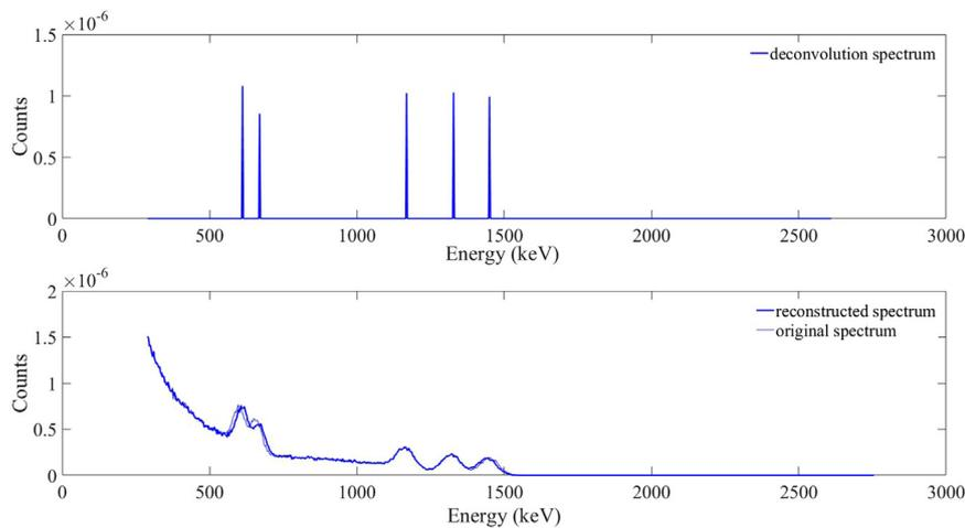
**Fig. 8.** Effect of the deconvolution method applied to the experimental spectrum for the radionuclide identification. The deconvolution spectrum for better radionuclide identification is shown in the upper part of the figure and below, the before-and-after experimental spectra are shown. Thin and thick lines show the original spectrum and reconstructed spectrum after deconvolution, respectively.
