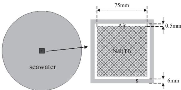
Fig. 5. Measurement simulation model of NaI(Tl) detector immersed in seawater.
