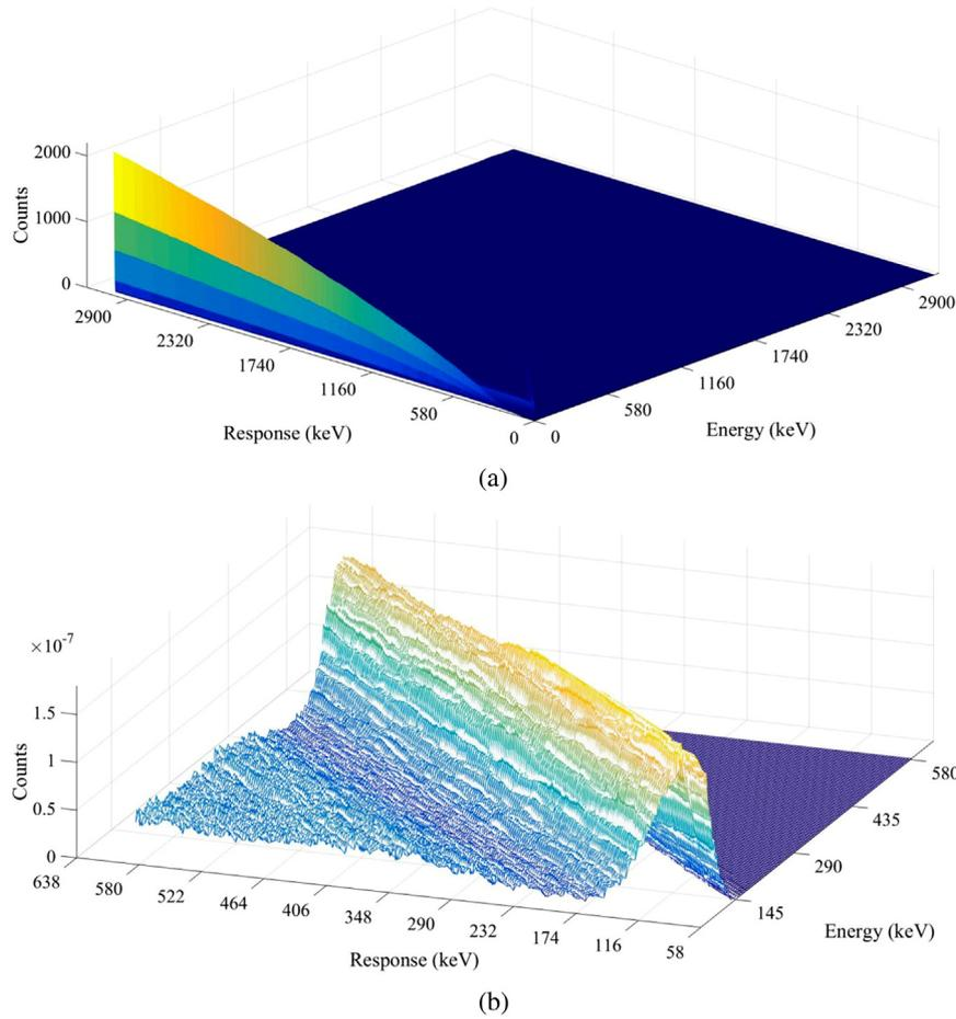
Fig. 7. The simulated response matrix. (a). the whole matrix. (b) the part of simulated response functions.
