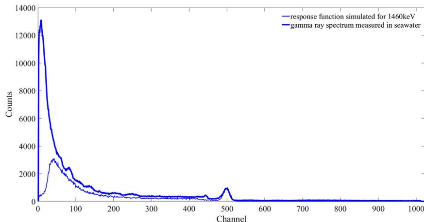
Fig. 6. Simulated spectrum for 1460 keV ( $^{40}\text{K}$ ) gamma ray contribution in the seawater in comparison with the spectrum measured in the field using NaI(Tl) detector developed. The measuring time is 34 h.
