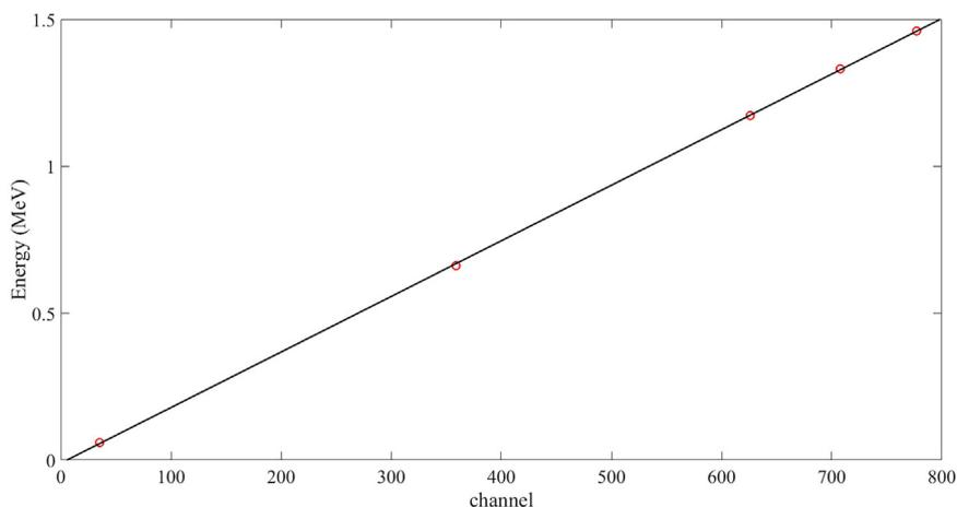
Fig. 2. Energy calibration curve of the detector by means of a set of radioactive point sources. The dots are experimental values. The solid line is a linear fit through the experimental points.
