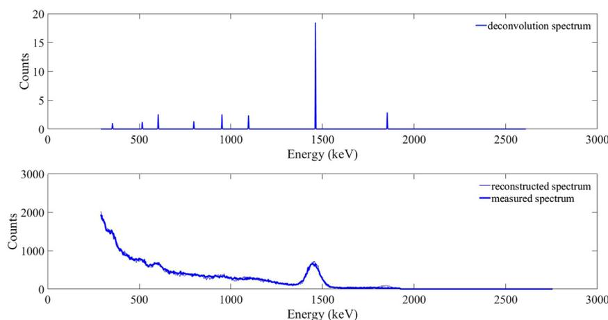
**Fig. 9.** Effect of the deconvolution method applied to the measured spectrum for the quantitative detection. The deconvolution spectrum for better detection is shown in the upper part of the figure and below, the before-and-after spectra in seawater are shown. Thick and thin lines show the original measured spectrum and reconstructed spectrum after deconvolution, respectively.
