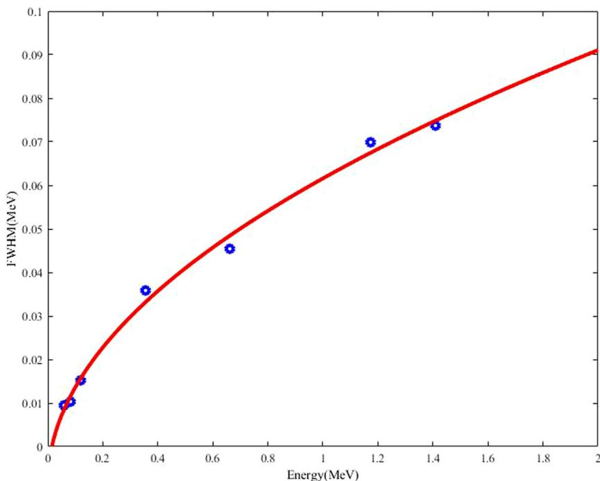
Fig. 3. Energy resolution calibration curve of the detector by means of a set of radioactive point sources. The dots are experimental values. The solid line is a fit through the experimental points.
