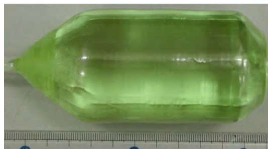
Fig. 1 2-inch-diameter bulk Pr:LuAG single crystal grown by the Cz method
