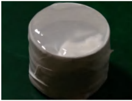
Fig. 4. The covered surfaces of the crystal by Teflon and the silicon grease.
