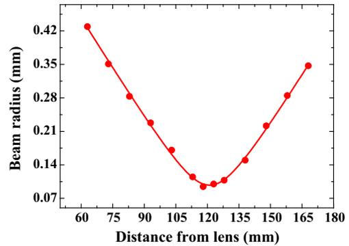
Fig. 6. The beam quality of the single-longitudinal-mode Ho:YLF ring laser.
