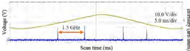
Fig. 4. The F-P spectra of unidirectional operation of the Ho:YLF ring laser.
