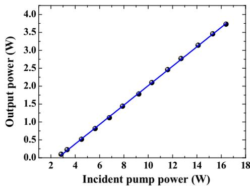
Fig. 5. The output power of the single-longitudinal-mode Ho:YLF ring laser.
