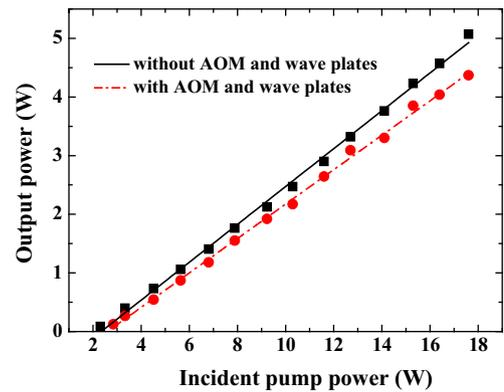
Fig. 2. The output power of the bidirectionally Ho:YLF ring laser.
