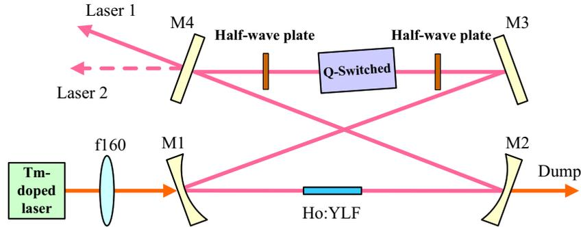
Fig. 1. The schematic of single-longitudinal-mode Ho:YLF unidirectional ring laser.
