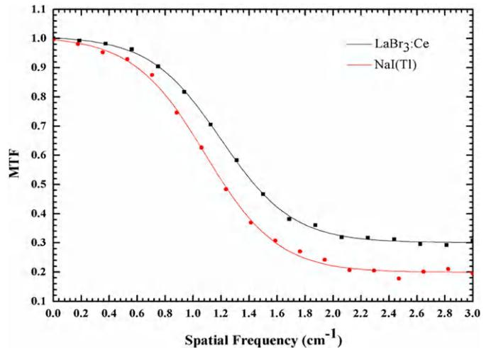
Fig. 3. Simulated MTF for the  $\text{LaBr}_3:\text{Ce}$ , and  $\text{NaI}(\text{Tl})$  crystal-based systems.
