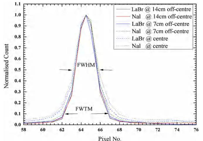
Fig. 4. Simulated horizontal profiles of  $^{99m}\text{Tc}$  point sources for the  $\text{LaBr}_3:\text{Ce}$  and  $\text{NaI}(\text{Tl})$  scintillators.
