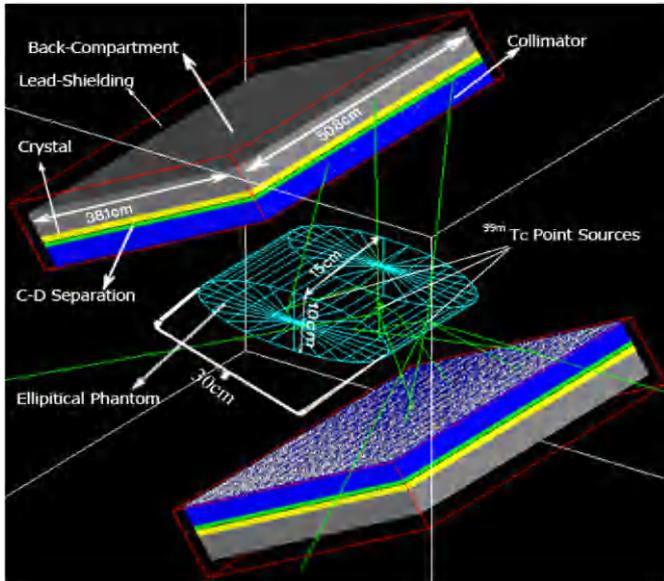
Fig. 1. A dual-head gamma camera and an elliptical Phantom as modelled by GATE.
