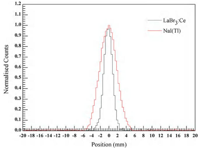
Fig. 2. Simulated PSF of a  $^{99m}\text{Tc}$  point source for the  $\text{LaBr}_3:\text{Ce}$ , and  $\text{NaI}(\text{Tl})$  scintillators.
