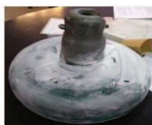
Fig. 3. artificially contaminated insulator
