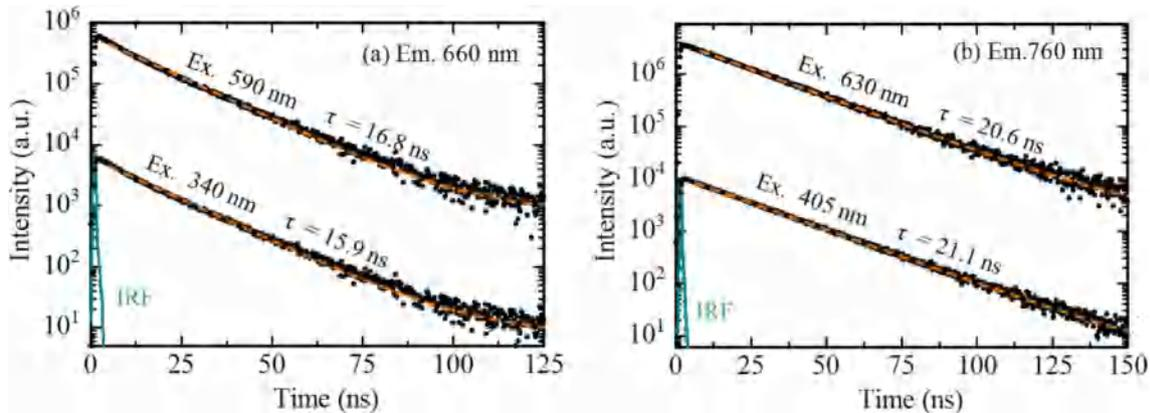
Fig. 3. PL decay time profiles monitored at (a) 660 nm under 340 and 590 nm excitations, and (b) 760 nm under 405 and 630 nm excitations with the instrumental response function.
