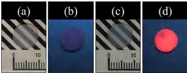
Fig. 1. (a) Non-irradiated and (c) irradiated samples under LED light, and (b) non-irradiated and (d) irradiated samples under UV light (365 nm).
