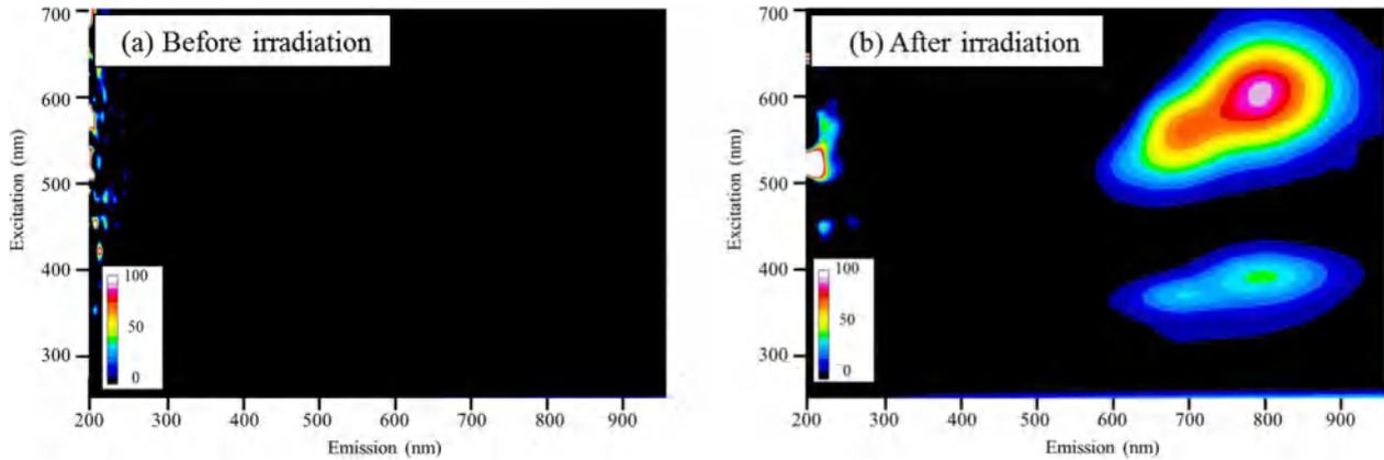
Fig. 2. PL excitation and emission maps of the (a) non-irradiated and (b) irradiated samples. The horizontal and vertical axes show emission and excitation wavelengths, respectively.
